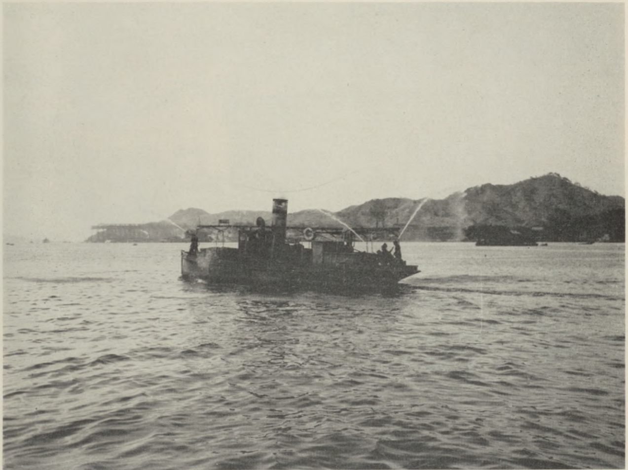
Photo 8. One of the two water police patrol boats, each equipped with a fire pump. Illustration shows two one-half-inch and one three-quarter-inch streams from a 350 g. p. m. pump driven by a Ford V-8 motor.
